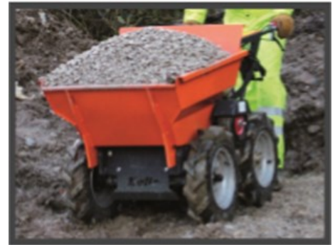
Large tray with a load capacity of up to 300 kg.
